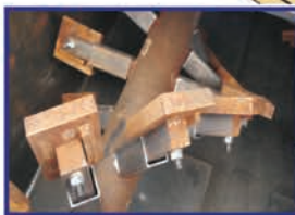
Bolt on Paddle Tips for Easy Replacement
